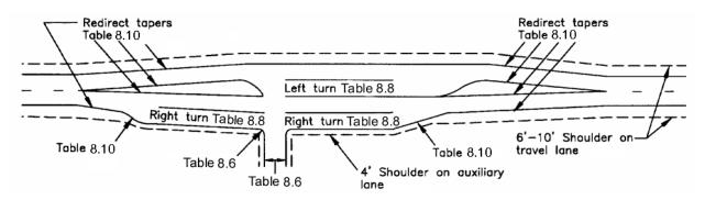
Figure 8.2—Information Guide to Basic Auxiliary Lane Elements
