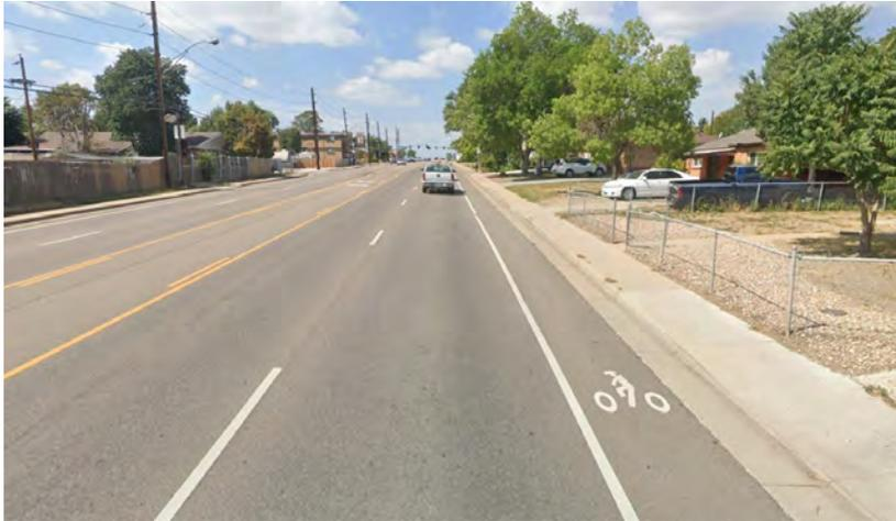
**Figure 10:** Example of a Bicycle Lane (88th Avenue at Downing Street)
