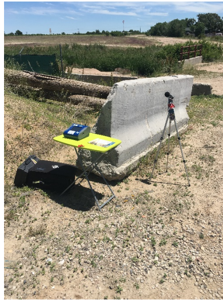
PM10 Sample # PME and Sound Level Monitoring Sample #SLME on the east perimeter of Henderson Pit (looking east, typical)
