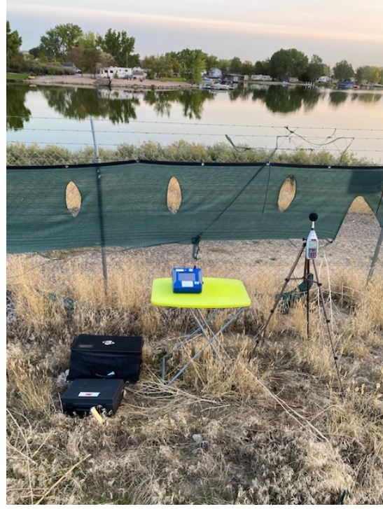
North Perimeter DustTrac and SLM
