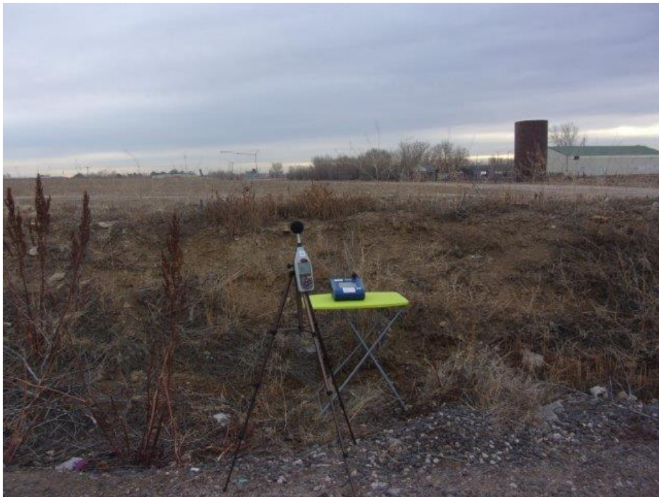
Sound Level Meter and Particulate Dust Monitor – East Perimeter Sample Location
