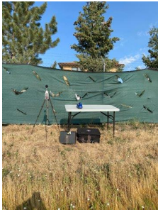
West Perimeter DustTrac and SLM
